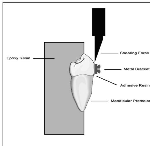
Figure 2. Mounting of sample.
