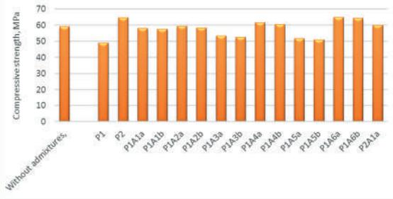
Figure 12. The compressive strength of mortars with different types of admixtures after 28 days
