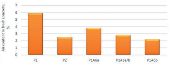
Figure 14. The air content in fresh concrete with different admixtures type
