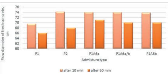
Figure 15. The flow diameter of fresh concrete with different admixtures type after 10 and 60 min
