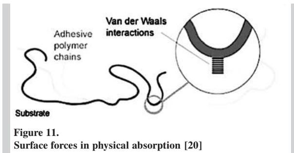
Figure 11. Surface forces in physical absorption [20]
