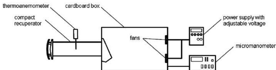
Figure 4. Scheme of air velocity distribution test stand
