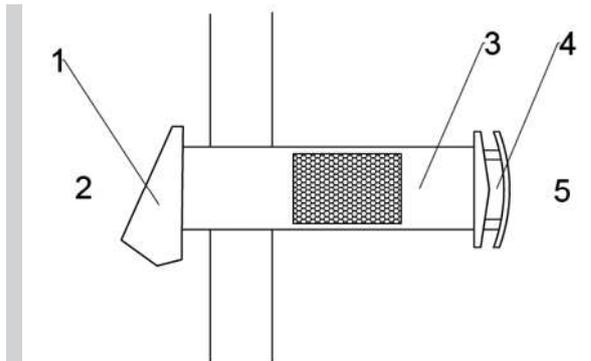
Figure 3. Location of the thermocouples; 1) in the air intake, 2) in the outdoor environment, 3) between the heat exchanger and the fan, 4) behind the fan (air inlet to the room), 5) in the room
