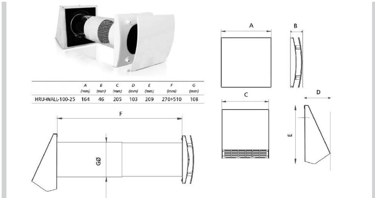
Figure 1. HRU-WALL-100-25 compact recuperator and its dimensions in millimeters [11]
