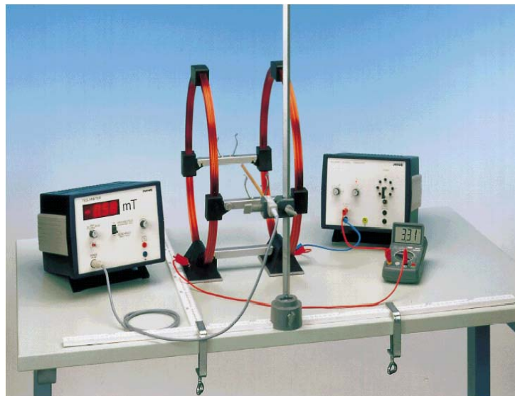
Fig. 12. The experimental set-up of Helmmoltz coil
