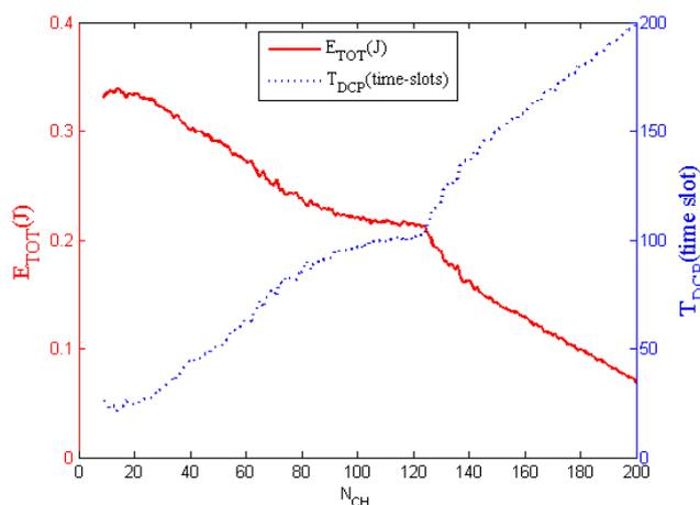
Figure 3, the simulation result of energy consumption and delay by leach in the area of  $2000 \times 2000 (m^2)$  and sink node is located at (1000, 1000).
