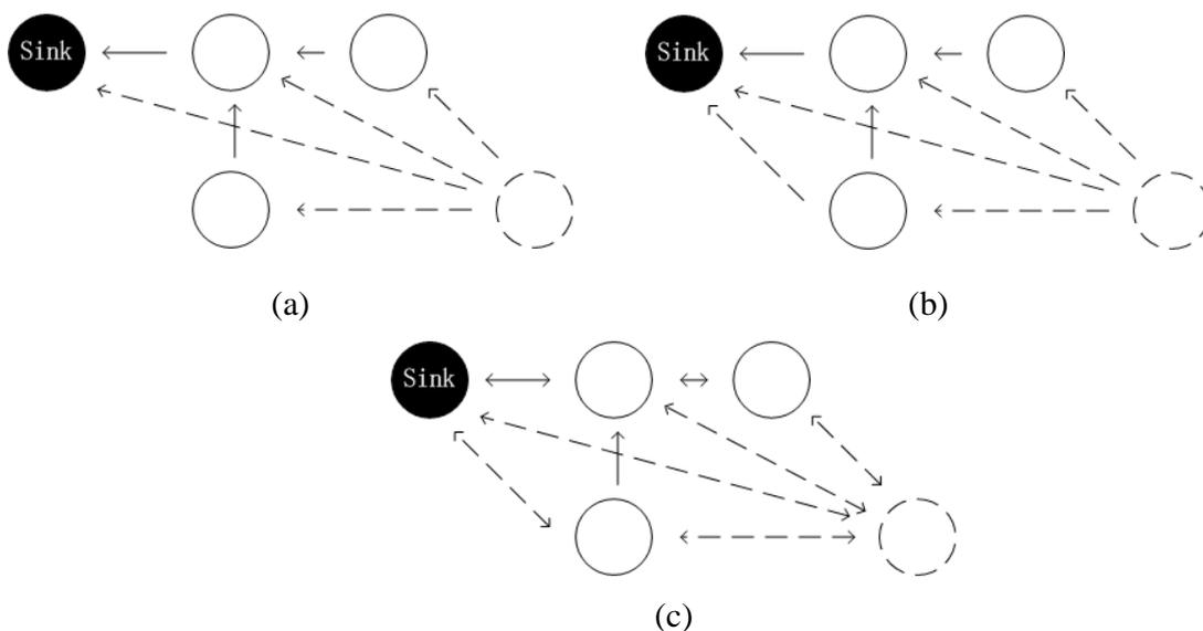
Figure 1. The description of connectivity in form of graphics: (a) Isolation nodes. (b) End-to-end connectivity. (c) Network connectivity.
