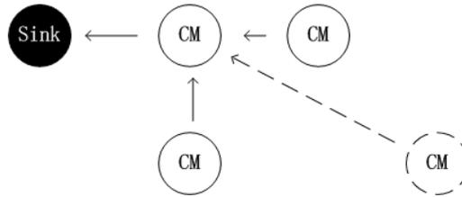
Figure 2. An example of isolation nodes in the cluster-based network
