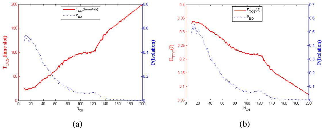
Figure 4. The simulation results by leach in the area of  $2000 \times 2000(m^2)$  and sink node is located at (1000, 1000): (a) delay and isolation nodes probability; (b) energy consumption and isolation nodes probability.
