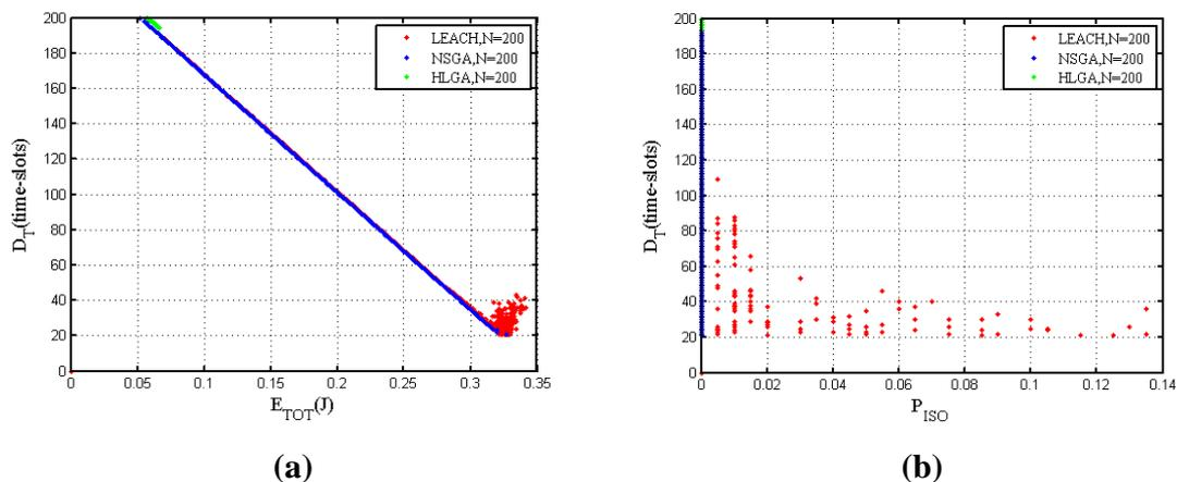
Figure 6. The simulation of different algorithms which contain Leach, NSGA and HLGA with  $200 \times 200 (m^2)$ : (a) The performance of energy consumption and delay; (b) The performance of delay and the probability of isolation nodes.
