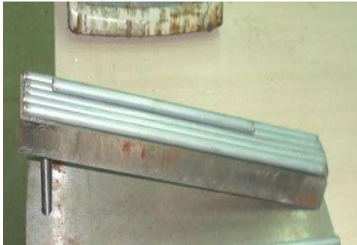
Figure 2. Friction coefficient test under the action of gravity
