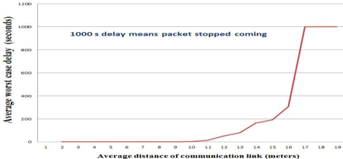
Figure 8: Avg. Delay vs. Avg. Distance, for multi hopping with constant distance throughout the network.
