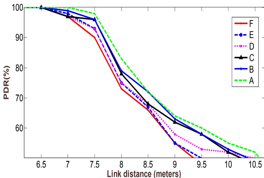
Figure 7: PDR vs. Distance for multi hopping with constant distance throughout the network for every node.
