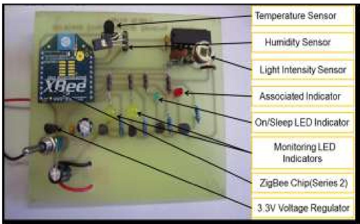
Figure 4: The fabricated sensor node with ZigBee.
