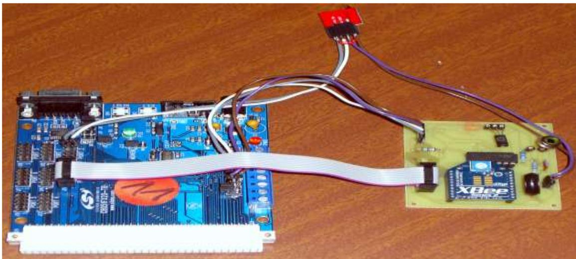
Figure 3: The developed system with ZigBee as only transceiver
