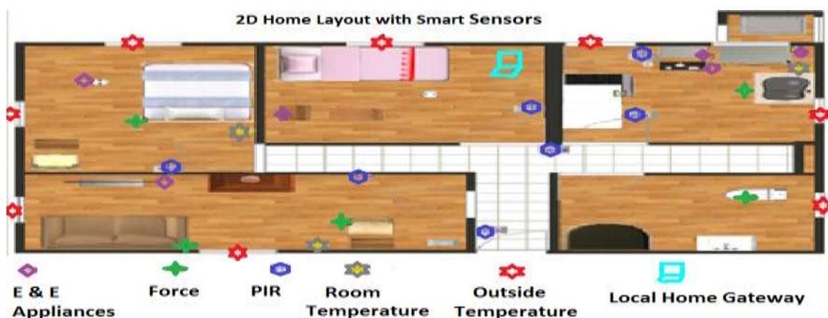
Figure 1: Placement of heterogeneous wireless sensor units using XBee (ZigBee) protocol in an old home.
