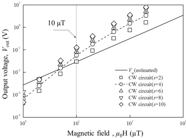
Figure 11. Output voltage of the CW circuit as a function of magnetic field strength. The frequency of magnetic field was  $60 \text{ Hz}$ .
