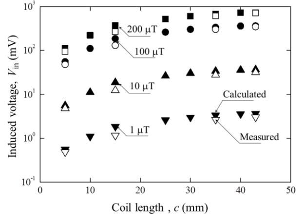
Figure 4. Induced voltage as a function of coil length, as a parameter of magnetic field strength. The frequency of magnetic field was 60 Hz.
