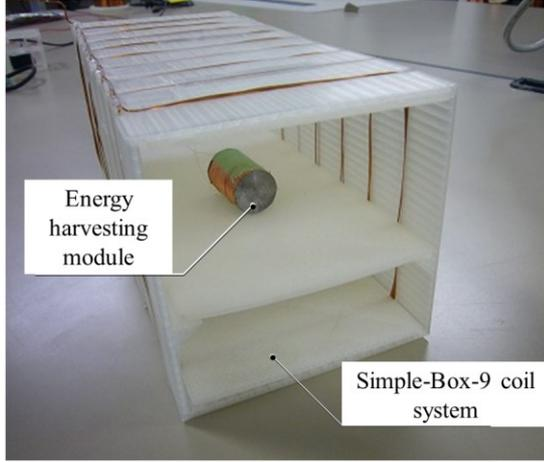
Figure 7. Experimental setup for evaluation of the energy harvesting module.
