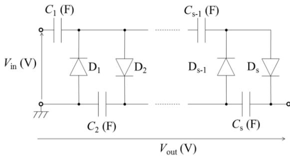
Figure 9. Schematic design of CW circuit.
