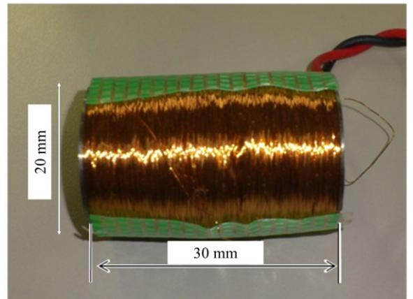
Figure 6. Energy harvesting module for magnetic field alarm. The magnetic flux concentration core was made of iron, whose flange length was 0.5 mm.
