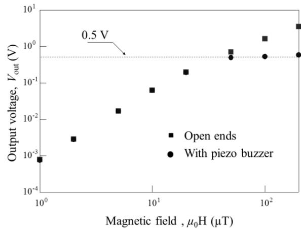
Figure 14. Measured output voltage as a function of magnetic field strength. The frequency of magnetic field was  $60 \text{ Hz}$ .
