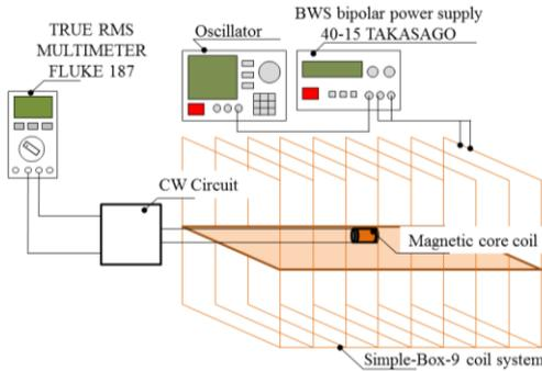
Figure 10. Experimental setup for evaluation of the CW circuit.
