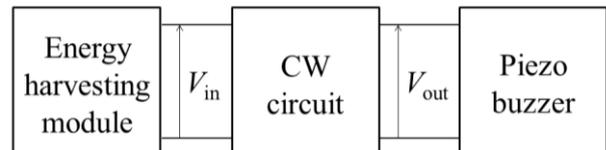
Figure 1. Schematic diagram of magnetic field alarm.
