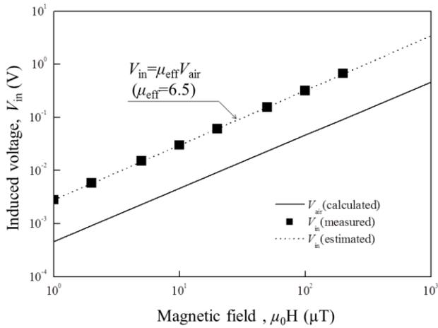
Figure 8. Induced voltage of the energy harvesting module as a function of magnetic field strength. The frequency of magnetic field was 60 Hz.
