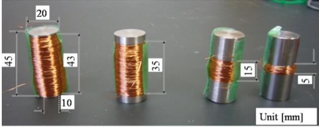
Figure 3. An example of energy harvesting modules as a function of the coil length. Magnetic flux concentration cores were made of PC permalloy.
