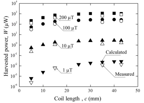
Figure 5. Harvested power as a function of coil length, as a parameter of magnetic field strength. The frequency of magnetic field was 60 Hz.
