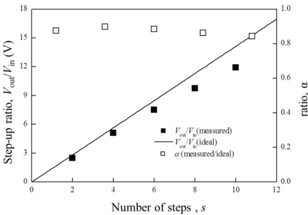
Figure 12. Measured ratios,  $V_{\text{out}}/V_{\text{in}}$  and  $\alpha$ , as a function of the number of steps in the CW circuit. Magnetic field was  $200 \mu\text{T}$  at  $60 \text{ Hz}$ .
