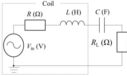
Figure 2. Equivalent circuit of the energy harvesting module.
