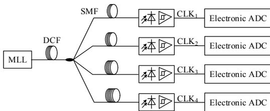
Figure 3. Architecture of the optoelectronic clock system for TIADC. MLL: mode locked laser. DCF: dispersion compensation fiber. SMF: single mode fiber.
