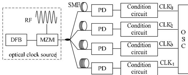
Figure 4. Experimental setup of the optoelectronic clock system for a two channel TIADC. DFB: distributed feedback optical source. MZM: Mach-Zehnder intensity modulator. SMF: single mode fiber. PD: photodiode. OSC: oscilloscope.
