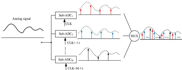
Figure 1. Structure of time-interleaved ADC system with  $M$  channels
