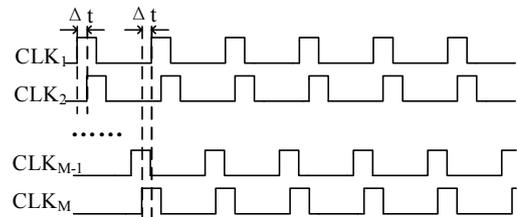
Figure 2. Staggered sample clocks for a time-interleaved ADC with  $M$  channels
