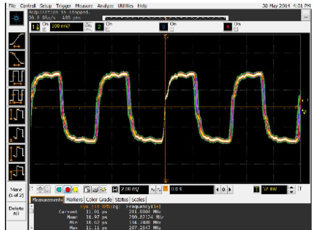
Figure 6. Eye diagram of the optoelectronic clock signal
