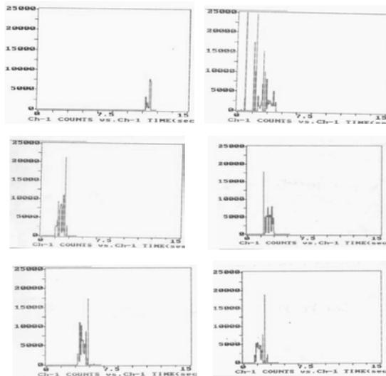
Fig. 11. AE Counts observed during end cap welding with defects generated by variation in weld parameters
