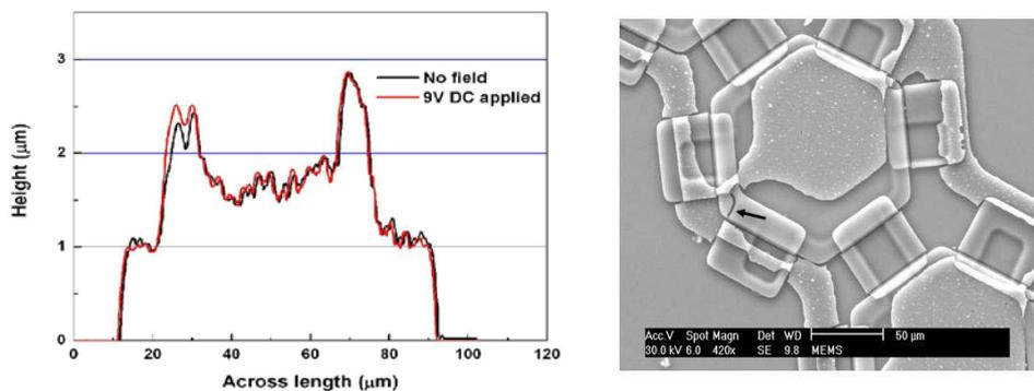
Fig. 5. Surface Profile Single cMUT Array. with and without field.
