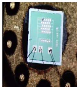
Fig. 4. . Packaged cMUT 5X5 and 5X1 array
