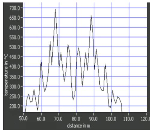
Fig. 2. Temperature measurement on the loop using RDTS
