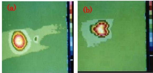
Fig. 10. Thermograms of (a) good weld and (b) of bad weld
