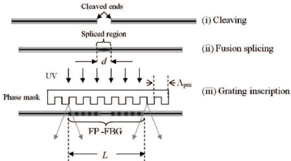
Fig. 3: The fabrication procedure of grating Fabry-Perot filter
