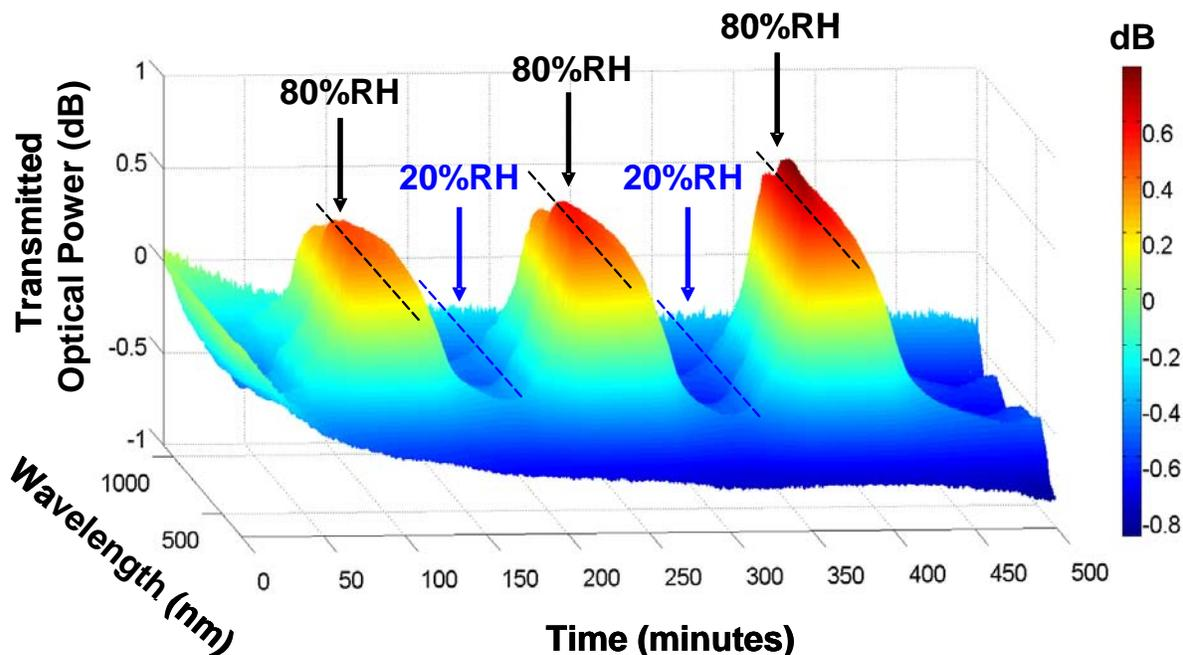
Figure 8. Spectral response of the sensor to changes in the RH (black arrow: 80% HR; blue arrow: 20% RH).
