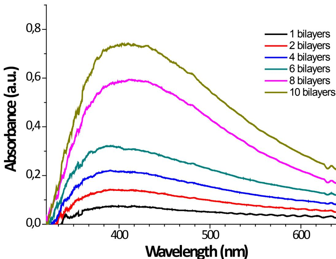
Figure 7. UV-VIS spectroscopy of the sensor as a function of the number of bilayers. The main absorption component is the SPR absorption band of silver NPs embedded into the polymeric film. The curves plotted are for 1, 2, 4, 6, 8 and 10 bilayers.
