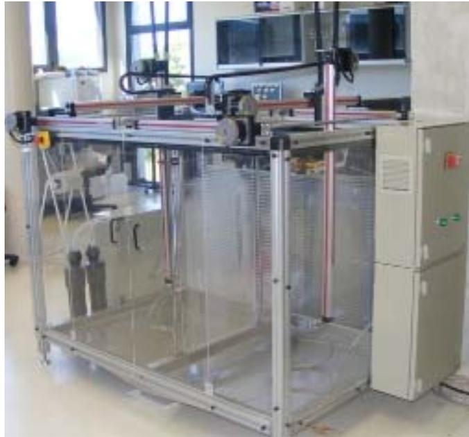
Figure 3. A 3-axis robot to the LbL process.
