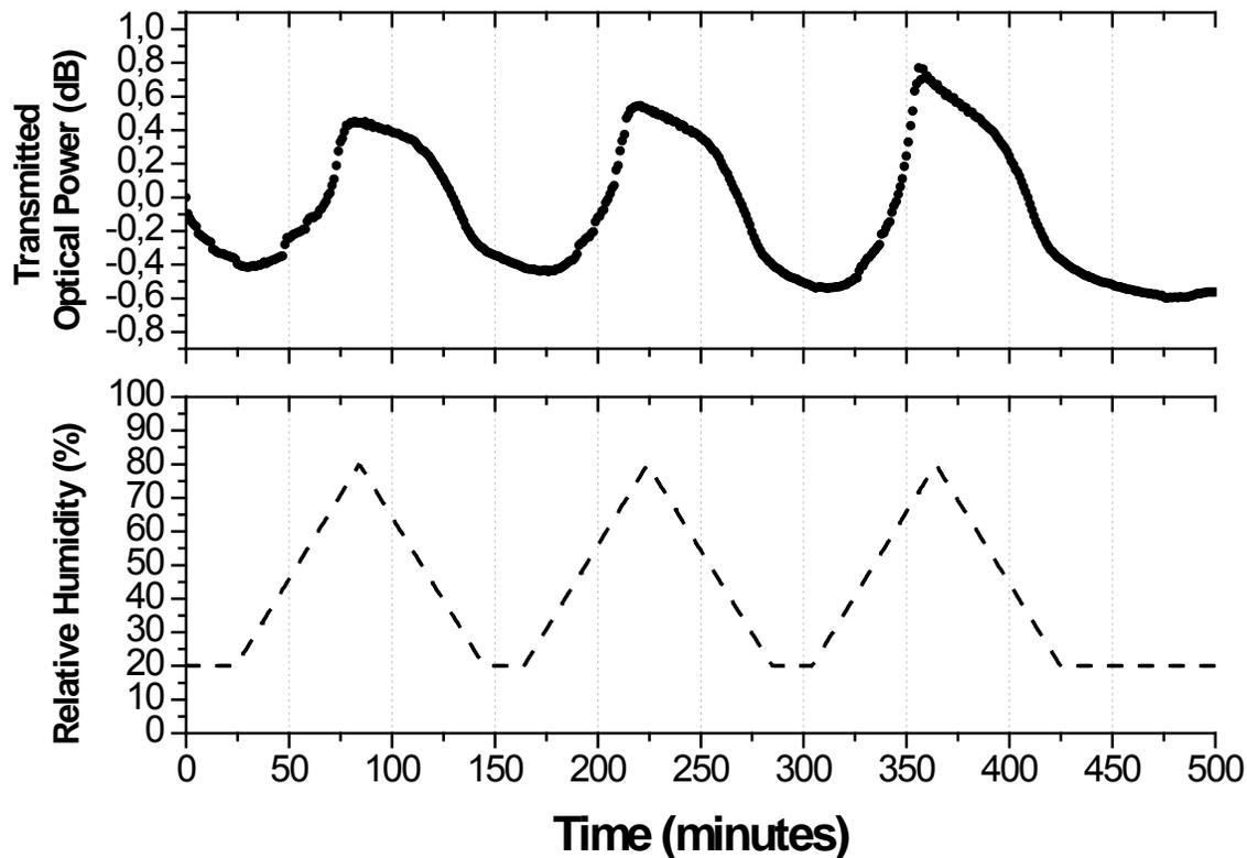
Figure 9. Optical fiber sensor response at 410 nm wavelength resonant peak (top) compared with the Set-Point Climatic chamber RH (bottom).
