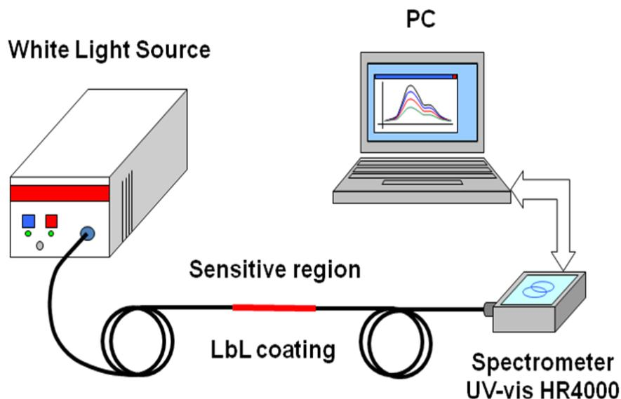
Figure 5. Schematic representation of the measuring setup.
