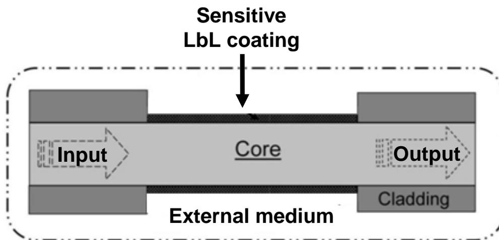
Figure 4. Detail of the sensitive region where LbL is deposited.
