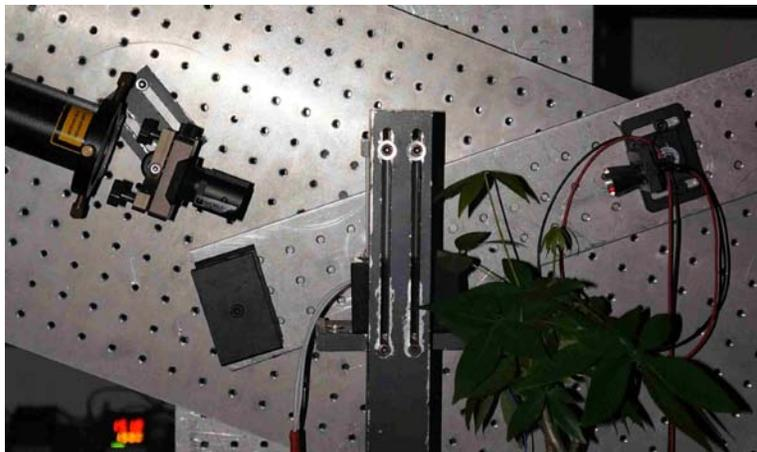
Fig. 3 The main frame of the temperature-controlled SPR in the setup of light response experiment.
