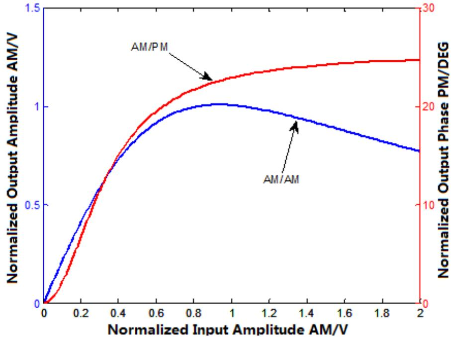
Figure 2.3: AM / AM and AM / PM Characteristic Curves of Model Saleh
