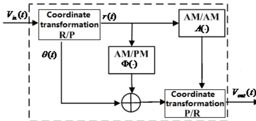
**Figure 2.1: General Form of Memoryless Nonlinear Model of Power Amplifier**
