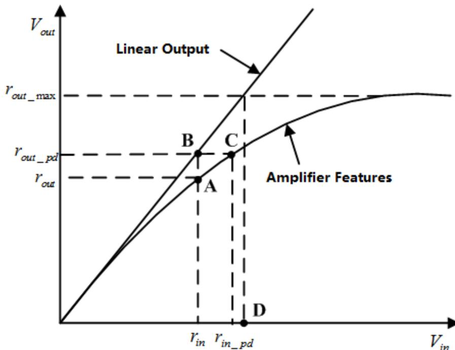
**Figure4.1: Schematic Diagram of Semi-automatic Pre-distorter**
