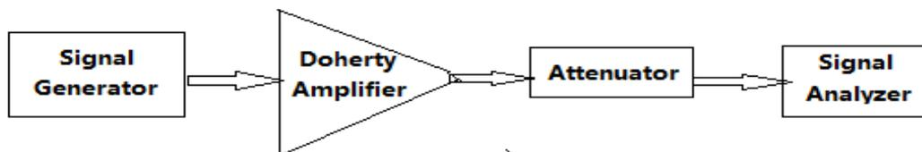
**Figure3.1: AM / AM Characteristic Measurement Block Diagram of Power Amplifier**
