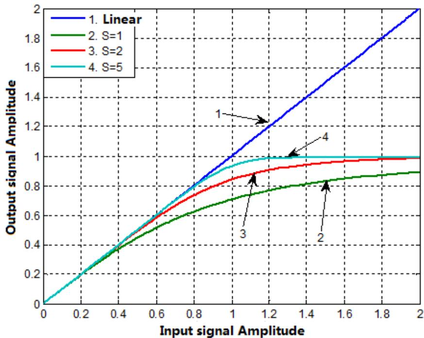
Figure2.2: AM / AM Characteristic Curve of Model Rapp Changing with Smooth Factor S
