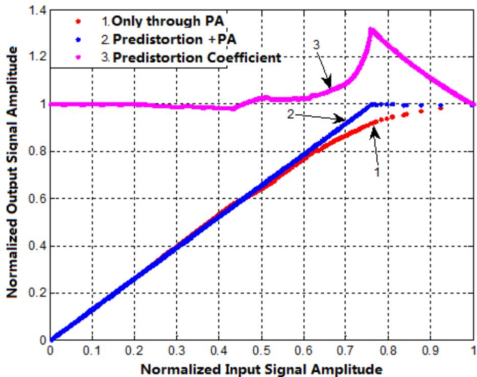
**Figure 4.2: Simulation Result of Semi-automatic Pre-distorter**
