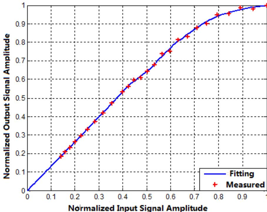
**Figure3.3: Characteristic Curve Fitting of Power Amplifier**
