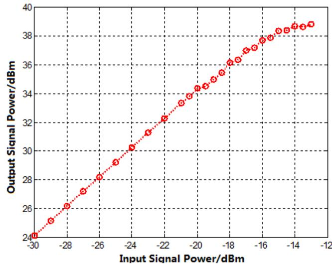
**Figure3.2: AM / AM Characteristic Curve of Power Amplifier**
