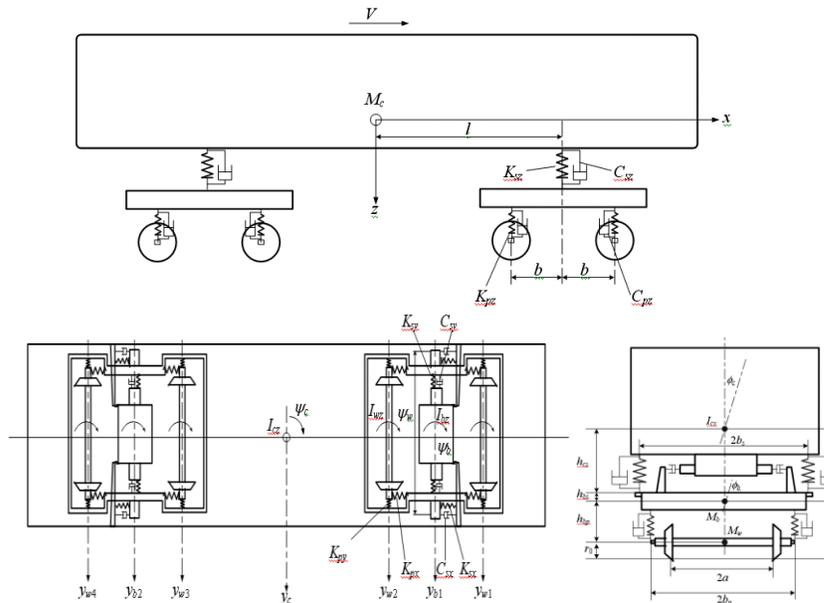
Figure 2. Lateral stability model for a vehicle
