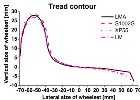
Figure 1. Contrast curve of the treads contour features
