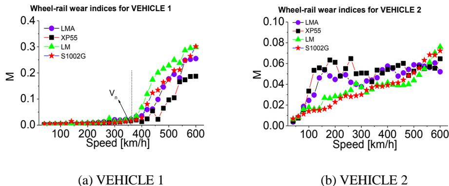
Figure 13. Normalized values of wheel-rail wear indices for VEHICLE 1 and VEHICLE 2 with different wheel-rail matching
