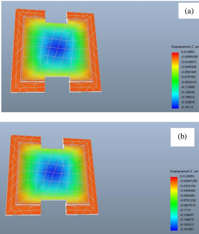
Fig. 5. Simulated view of the diaphragm displacement with applied pressure of (a) 0.3 kPa (b) 2 kPa
