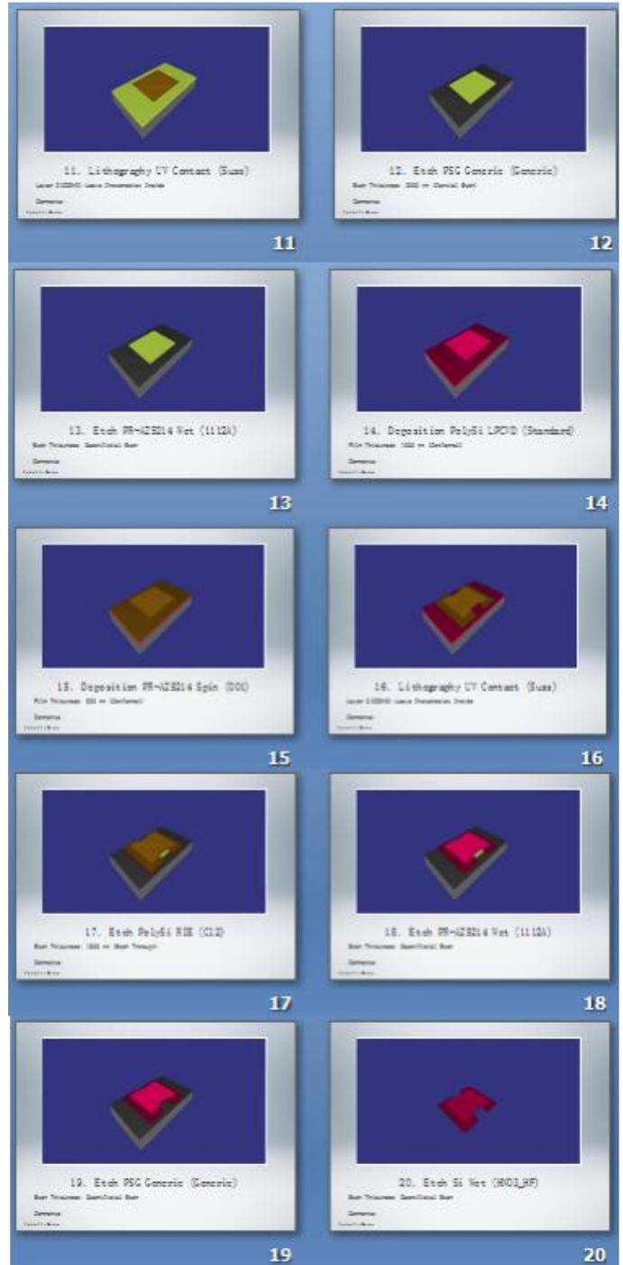
Fig. 3. Views of the virtually fabricated sensor with the above mentioned steps.
