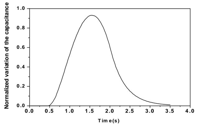
Fig. 8. Dynamic response of the diaphragm
