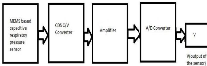
Fig. 9. Block diagram of the electronic system design architecture of the MEMS capacitive type nasal exhalation sensor
