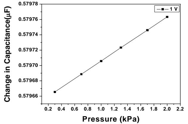
Fig. 7. Plot of Change in capacitance (μF) vs. Pressure (kPa)
