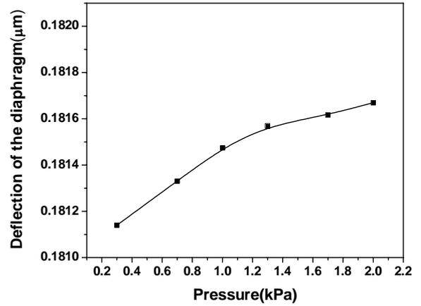
Fig. 6. Plot of deflection of the diaphragm corresponding to the pressure (0.2-2.2 kPa)
