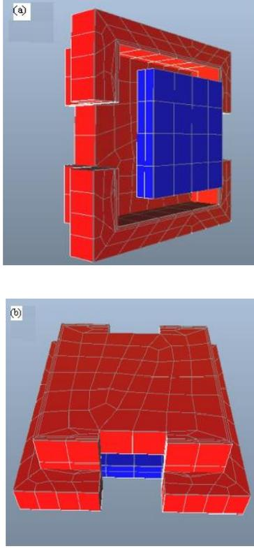
Fig. 2. 3D view of the designed respiratory sensor (a) Top view and (b) Side View
