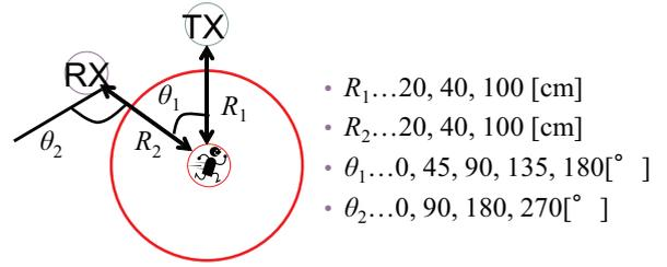
Fig. 8. Setup for collecting ultrasonic communication data.
