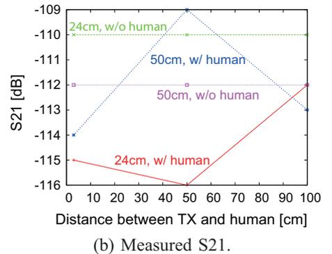
Fig. 6. Experiments for horizontal reflection.
