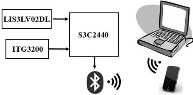
Figure 2. The hardware configuration diagram of the system
