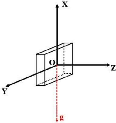
Figure 4. The sensor coordinate system.
