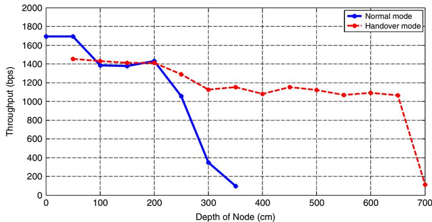
Figure 8: Throughput vs. depth in normal mode and handover mode.
