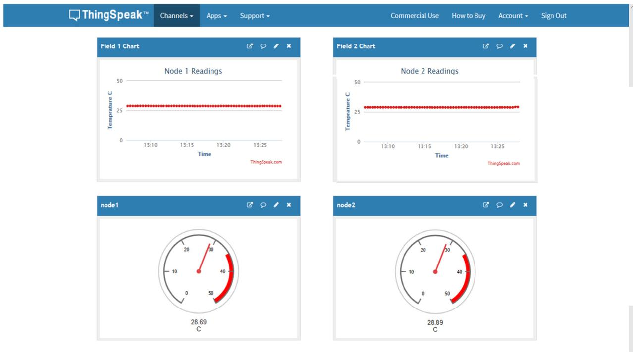
Figure 7: ThingSpeak platform visualization for temperature measurements under normal mode.
