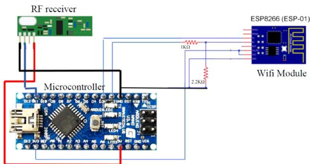
Figure 1: Server node schematic. The RF transceiver is used for UWC, while the Wi-Fi module is used for communication with the server.
