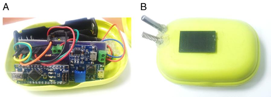
Figure 4: (A) Printed circuit board used in combining RF modem, (B) modem final form showing the antenna, the temperature sensor, and the solar cell.
