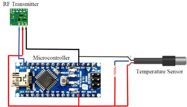
Figure 2: Terminal node schematic. The temperature sensor is used to collect data to be sent of the server.
