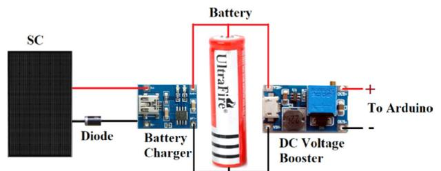
Figure 3: Solar charging circuit connection. The circuit is used to self-power the underwater node.
