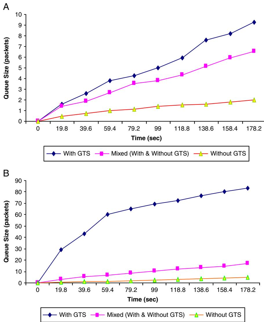
Figure 7: Queue size (A) PAN coordinator (B) End device.
