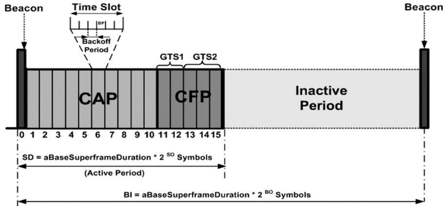
Figure 2: Superframe structure (Koubaa et al., 2007).
