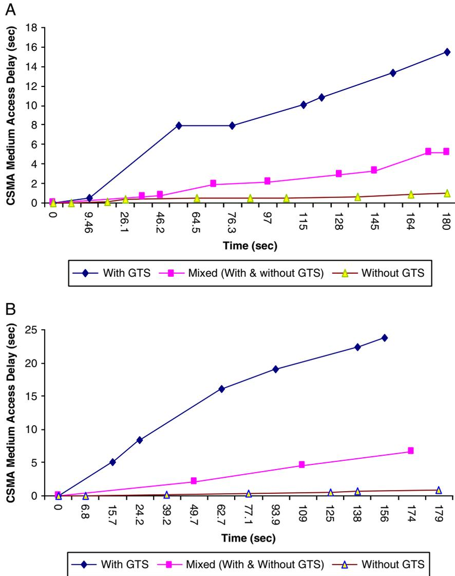
Figure 5: CSMA medium access delay: (A) PAN coordinator (B) End device.
