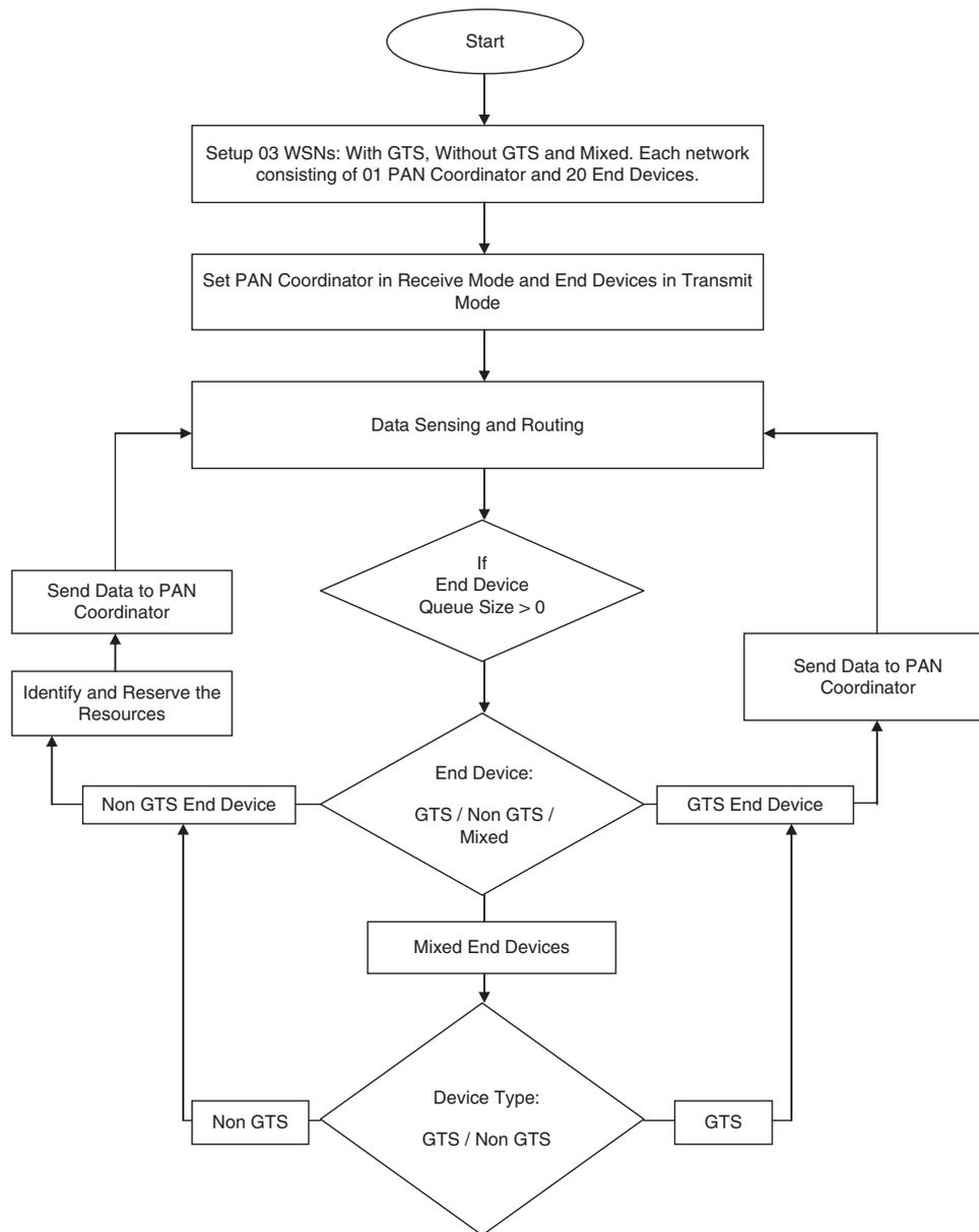
Figure 3: Flow Chart: Working of GTS, non-GTS, and mixed sensor networks.
