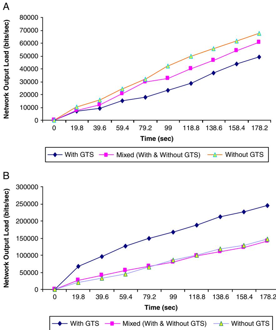
Figure 4: Network output load: (A) PAN coordinator (B) End device.
