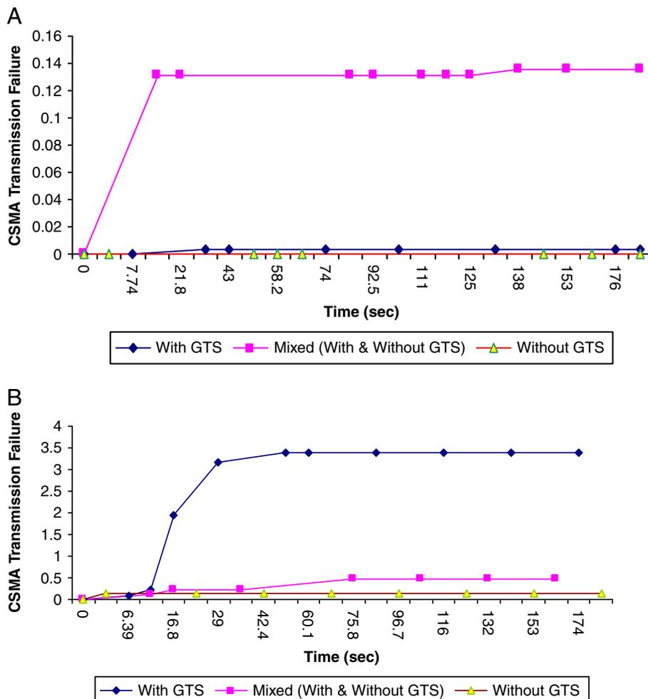
Figure 6: CSMA transmission failure (A) PAN coordinator (B) GTS end device.
