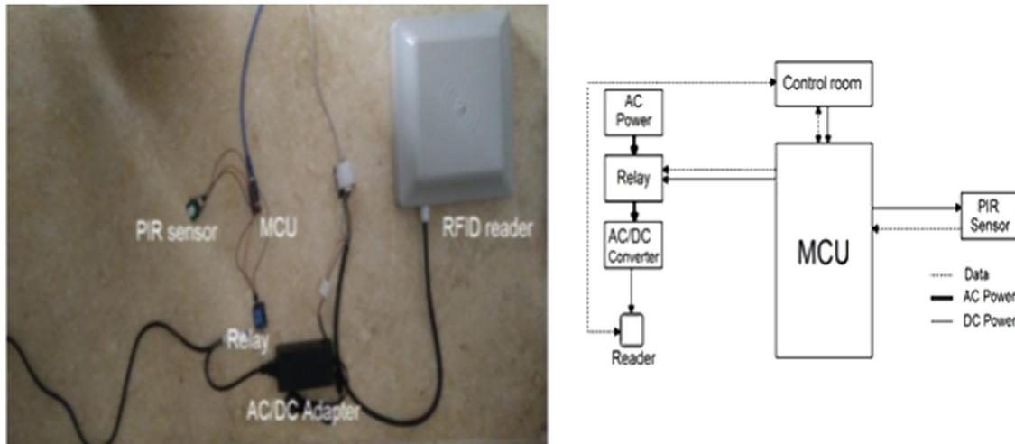
Figure 6: Implementation of the optimal motion sensor-based smart RFID system.
