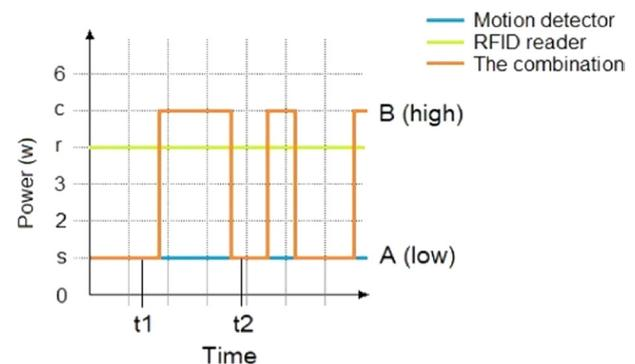
Figure 2: Illustrative representation of power consumed by RFID reader, motion detector, and their combination.
