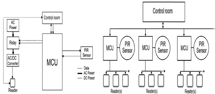
Figure 4: Block diagram of smart RFID system and a grid of smart RFID systems.
