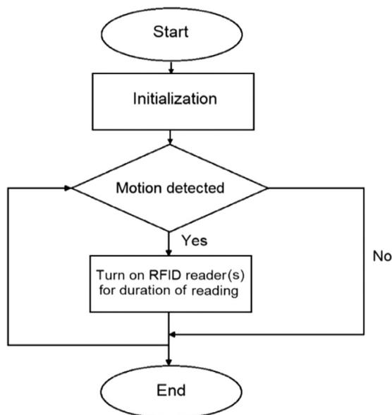
Figure 5: Program flowchart of PIR sensor-based RFID system.
