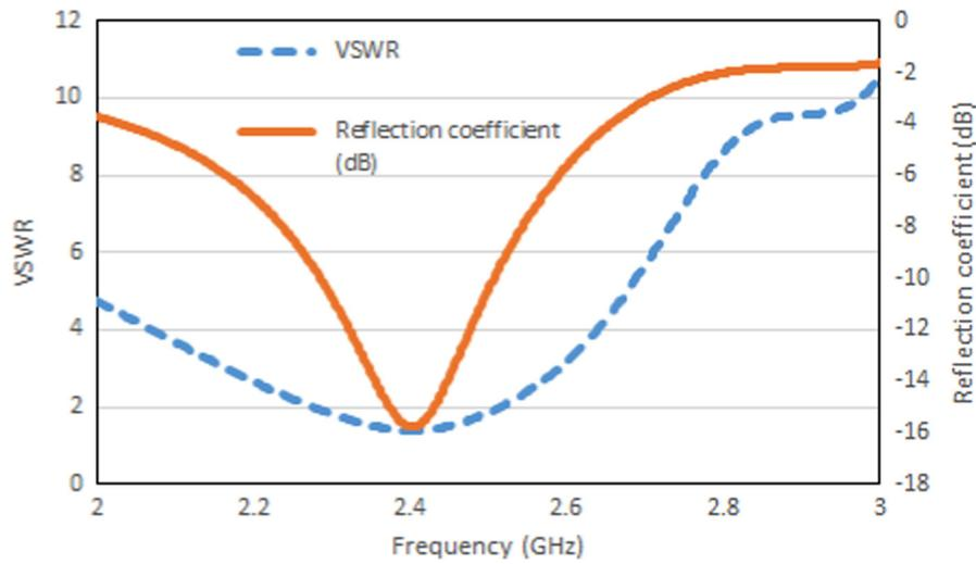
Figure 3: VSWR and reflection coefficient of the antenna.
