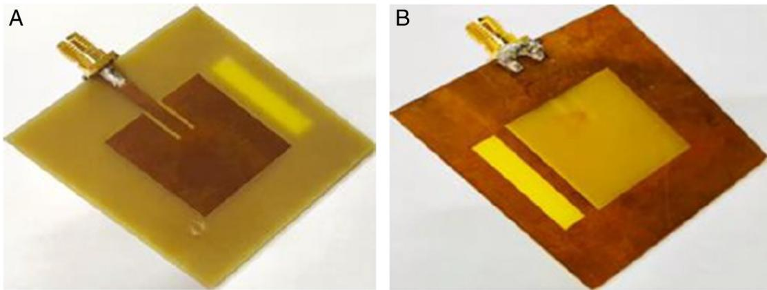
Figure 2: Fabricated antenna: (A) top view and (B) bottom view.
