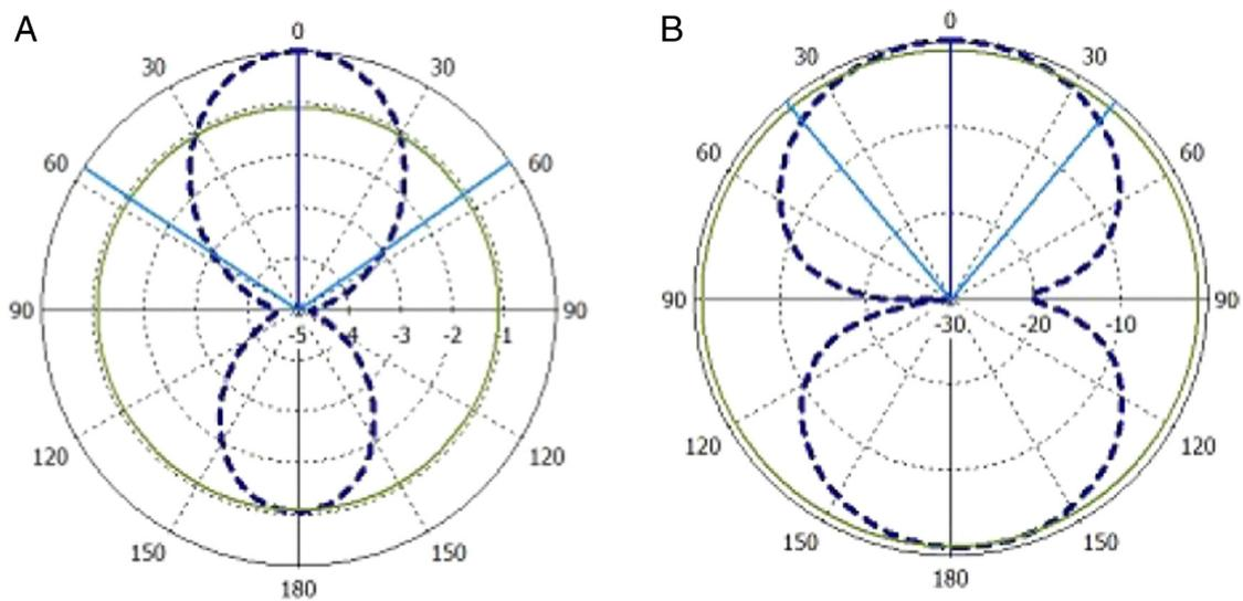
Figure 4: Radiation patterns of the antenna at 2.4 GHz: (A)  $\phi = 0$  deg. plane and (B)  $\phi = 90$  deg. plane.
