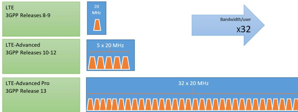
Figure 1: Carrier aggregation of up to 32 CC in LTE A PRO.
