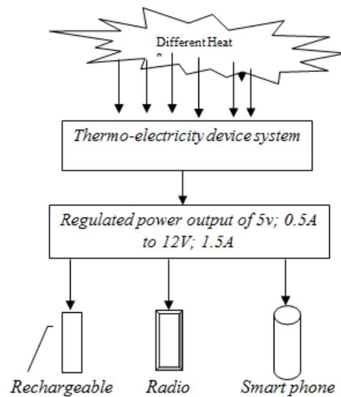
Figure 1. Operational arrangement of heat-to-electrify charger device.
