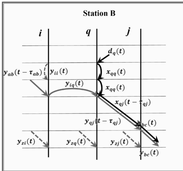
Fig. 1. Locomotive and makeup connection scheme:  $i$  – input sector,  $j$  – output sector,  $q$  – makeup origin point
