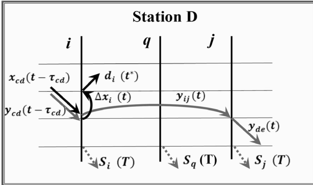
Fig. 3. Scheme of a train arrival at the terminal station:  $\Delta x_i(t)$  – delay
