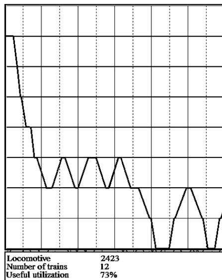
Fig. 6. Locomotive turnover schedule (the black line shows the idle time and empty running)
