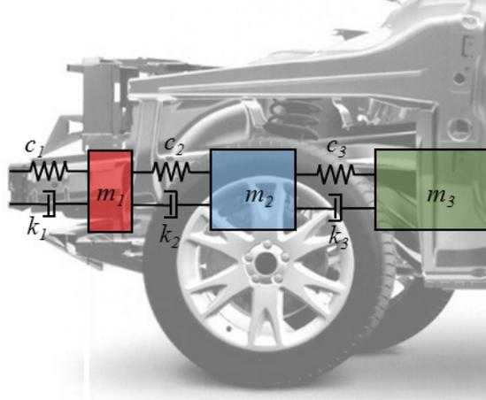
Fig. 1. Three-mass model for the front crumple zone
