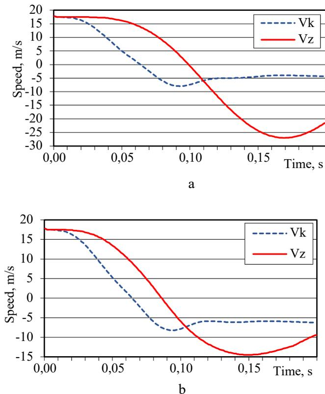
Fig. 18. Dependence of occupant's body ( $V_z$ ) and vehicle body ( $V_k$ ) speed in case of the impact at the speed of 64 km/h: a – without the safety system damping, b – with the safety system damping
