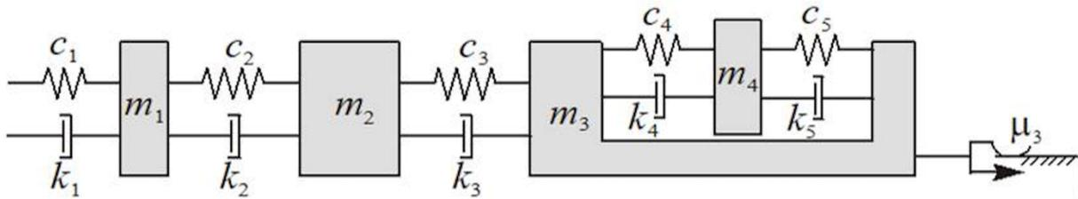
Fig. 9. Four-mass model for the front crumple zone
