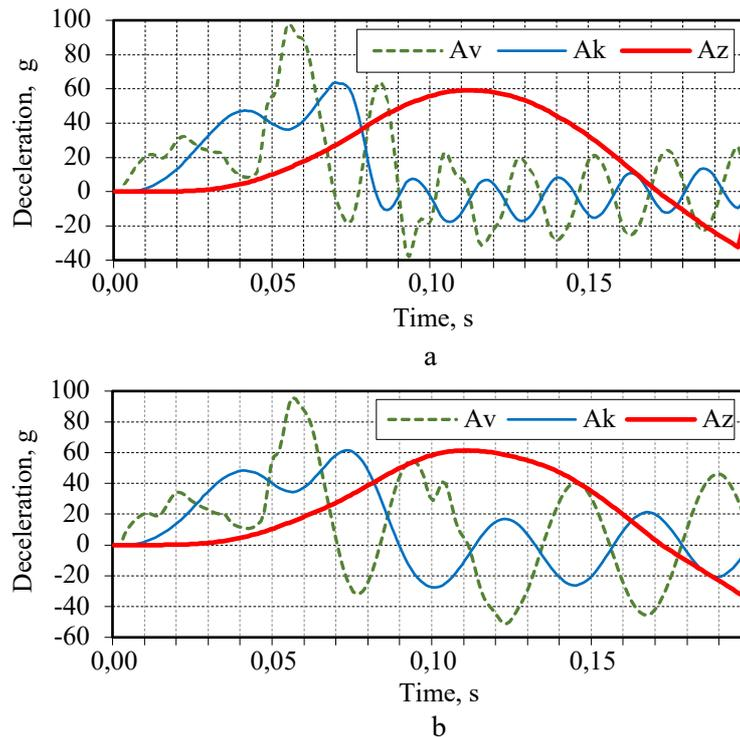
Fig. 17. Dependence of deceleration of vehicle engine zone ( $A_v$ ), vehicle body ( $A_k$ ), occupant’s body ( $A_z$ ) in case of an impact at the speed of 64 km/h, where the damping coefficients for zone 2: a - 1.3, b - 2.6.
