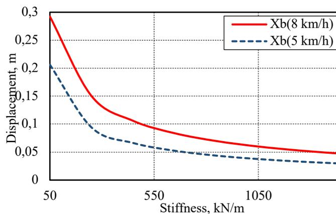
Fig. 7. Dependence of bumper displacement on bumper stiffness
