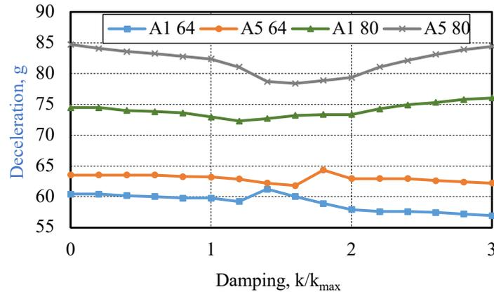
Fig. 16. Dependence of deceleration values in case of the impact at 64 and 80 km/h on the damping; where A1 and A5 – respectively, one and five occupants
