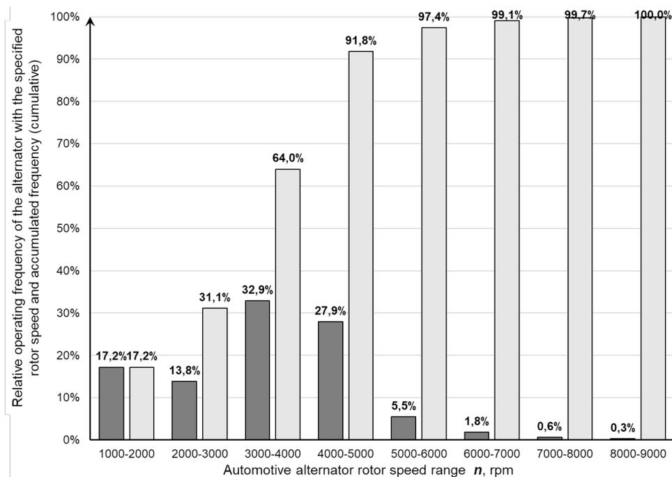
Fig. 3. Distribution of the Automobile Alternator Rotor Speed (the dark columns show the relative operation frequency and the light columns show the accumulated frequency (cumulative curve))
