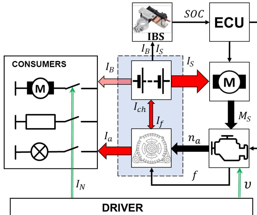
$I_S$  – starter current;  $I_G$  – alternator current;  $I_f$  – alternator excitation winding current;  $I_B$  – battery current;  $I_C$  – battery charge current;  $I_N$  – consumer (load) current;  $M_S$  – starter rotation torque;  $n_a$  – automobile alternator rotor speed;  $f$  – frequency signal about combustion engine operation; and  $v$  – automobile driving speed.
