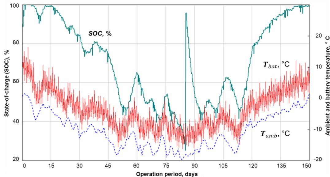
Fig. 1. Change in charge state and Temperature of the Battery during the Daily Operation of a Hyundai Solaris within the Period from November to March in Tyumen: SOC (state-of-charge) battery, %;  $T_{bat}$  – battery temperature, °C; and  $T_{amb}$  – ambient temperature, °C
