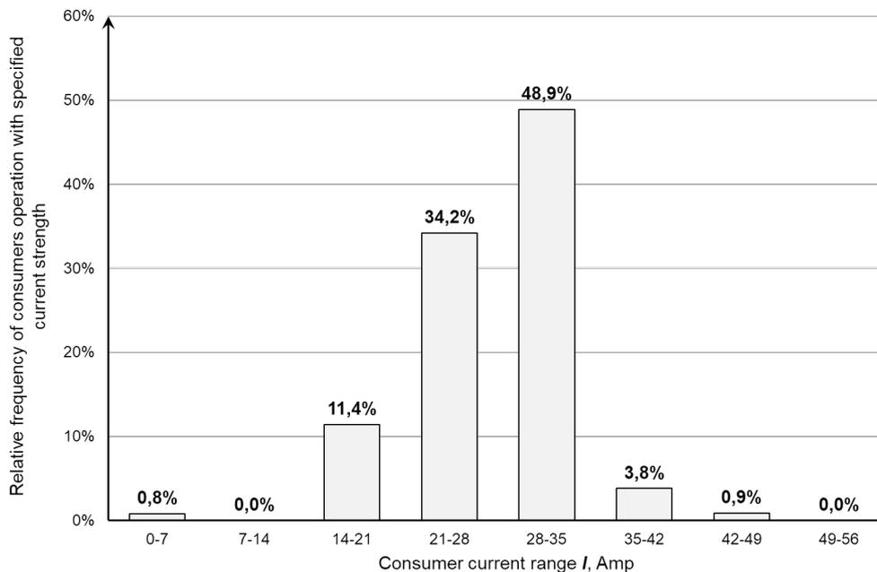
Fig. 4. Distribution of the current intensity of a passenger vehicle in urban traffic at night in winter
