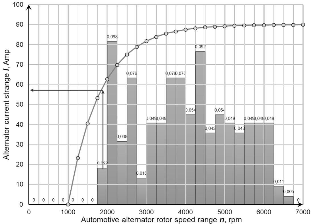
Fig. 2. Current and Speed Characteristics and Time Distribution of the Automobile Alternator Operation
