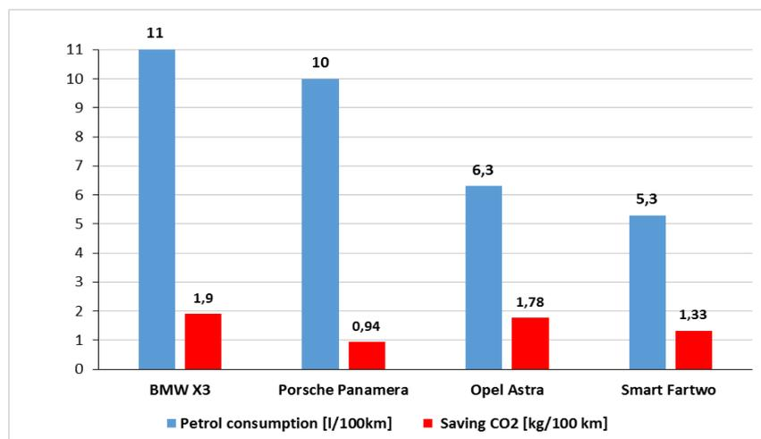
Fig. 3. Reduction emission of CO<sub>2</sub> with activated start–stop function
