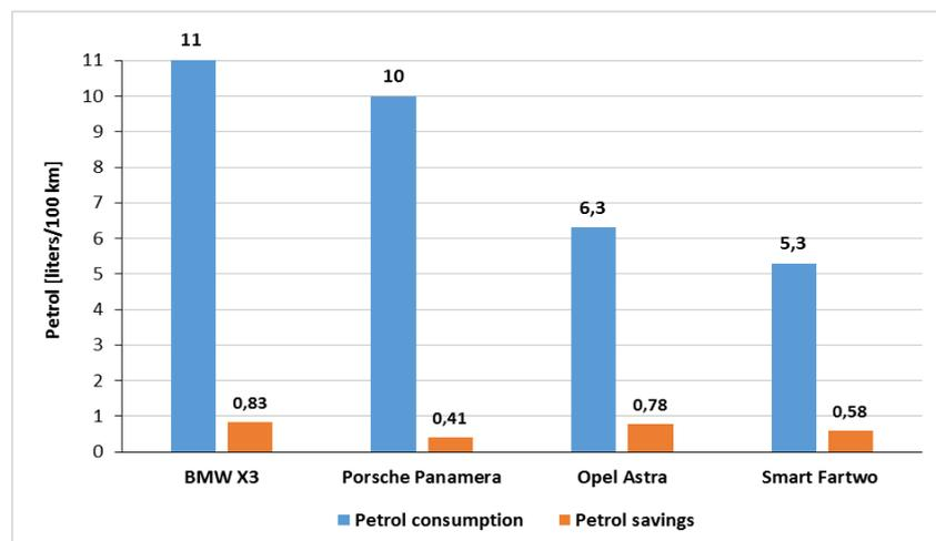
Fig. 2. Reduction of fuel with activated start–stop function
