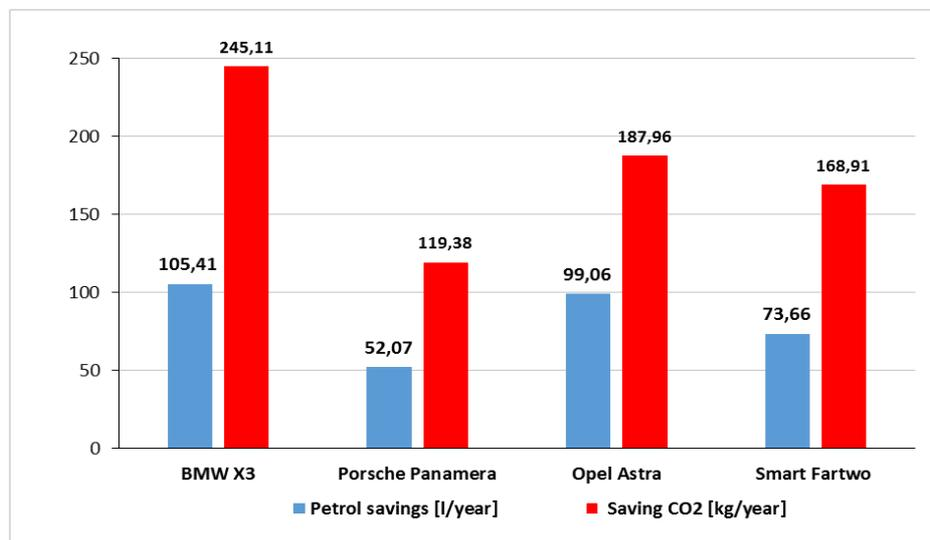
Fig. 4. Annual reduction of fuel and emission of CO<sub>2</sub> with activated start–stop function
