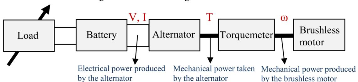
Fig. 1. Test bench configuration, where: V, I is the alternator voltage and alternator current, T is the alternator torque and  $\omega$  is the brushless motor rotational speed
