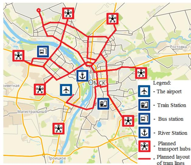
Fig. 1. Layout of transport facilities and perspective of their development
